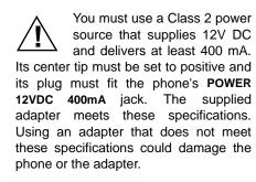
Always connect the AC adapter to the phone before you connect it to AC power. When you finish, disconnect the adapter from AC power before you disconnect it from the phone.
